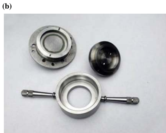
Fig. 3 (a) Design of gas permeability cell. (b) Photograph of gas permeability cell components
